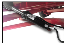
Cushion Cylinder With Adjustable Flow Valve
