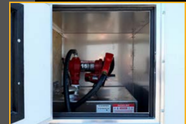
Built in 50-Gallon Fuel Tank
