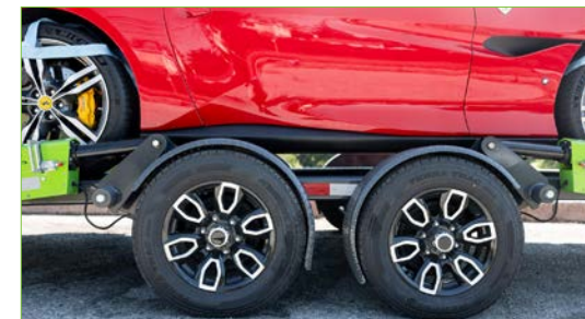
Fully upright position allows doors to clear wheel wells
