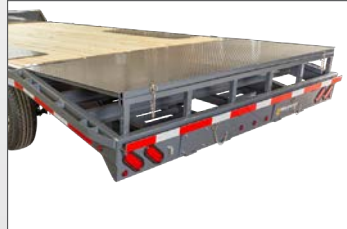
ADJUSTABLE BEAVERTAIL WITH 5' SLIDE IN LADDER RAMPS
