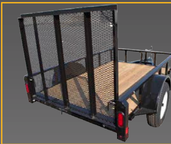
Tubular Frame Mesh Ramp with Spring Assist
