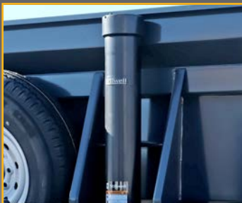
Low Profile 5-Stage Front Telescopic Cylinder
